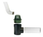
**TIP:** Dig the hole for the basin an additional 6" deeper than needed. Place 6" of gravel in the bottom of the hole. Drill small holes in the bottom of the basin to prevent standing water in the bottom of the basin, eliminating a potential mosquito breeding area.
