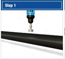
Place the saddle on a desired location and mark. Remove saddle, drill hole and deburr.
