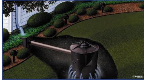
**Pop-Up Emitter** – Acting as the discharge point of a drainage system, Pop-Up Emitters release water from the drain pipe away from structural foundations in order to help manage water overflow. A spring-loaded cap opens when it senses the hydrostatic pressure of water flowing through the pipe, and it closes again when the flow decreases. The pop-up style keeps rodents and debris out of the system, and the low-rise height won't get in the way of mowers.
